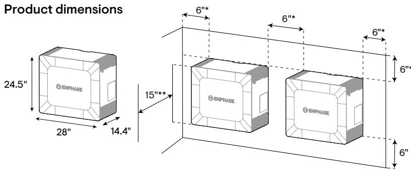
\* The 6 in clearances on the sides and the top are per the UL 9540A evaluation. Enphase recommends 8 in for ease of service.
